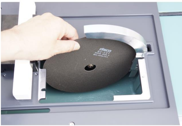
Exchanging blade(with the special vice)
