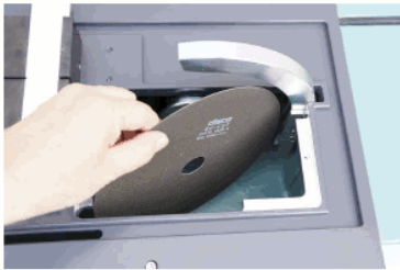
Replacement of a blade (with a special vise)
