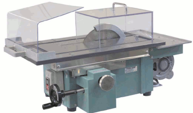
Example of cover installation
