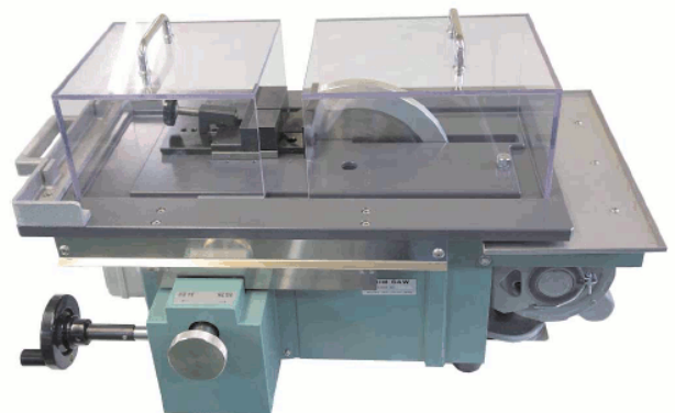
Front and rear covers when processing long workpieces
